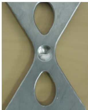
Figure 24: Typical fatigue failure of the biaxial specimen in Al 2024
