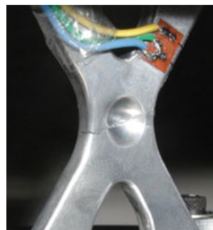
Figure 25: A biaxial fatigue specimen made from cast AlSi7-Cu0.5Mg0.3 showing that crack initiation did not occur in the biaxial zone in the centre of the specimen
