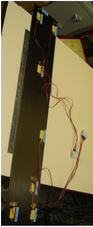
Figure 8: CLAS bounded with piezoceramic patches
