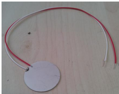
Figure 3: PZT disc from NOLIAC
