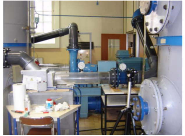
FIG. 4. Scheme of the DynFluid axial pump test-ring
