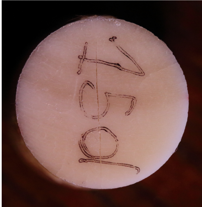
Figure 5: Appearance of a vertical crack at the centre of a specimen x_1\_F_3 with a 8.12 mm diameter.
