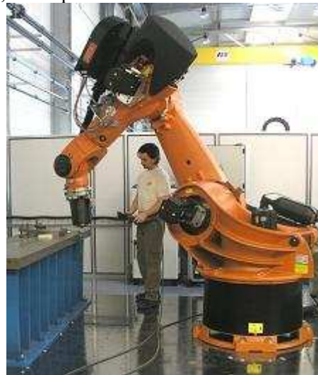
Figure 1: Serial kinematic robot for FSW application
