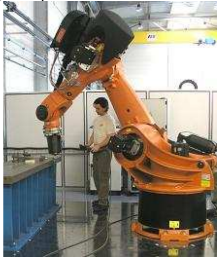
Figure 1: Serial kinematic robot for FSW application
