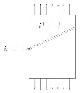
Fig. 9. Volume fraction of localized grains during a tensile test.
