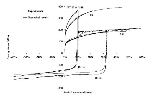
UT stands for Uniaxial Tension, BT for Bauschinger Test, SSh for Simple Shear and PT 10% SSh for Plane Tension until 10% of logarithmic strain followed by Simple Shear.
