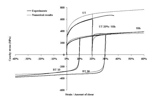
UT stands for Uniaxial Tension, BT for Bauschinger Test, SSh for Simple Shear and UT 20% SSh for Uniaxial Tension until 20% of logarithmic strain followed by Simple Shear.
