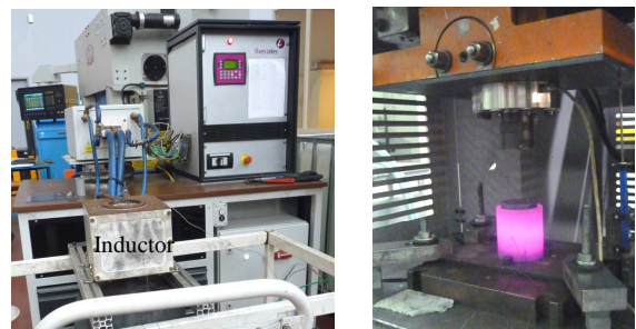
Fig.2 Induction heating system (left), and thixo-extrusion test device mounted on the press (right)
