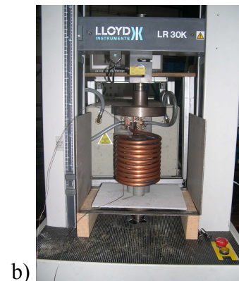
Fig. 1 a) Induction heating process scheme; b) Extrusion device on the Lloyd press
