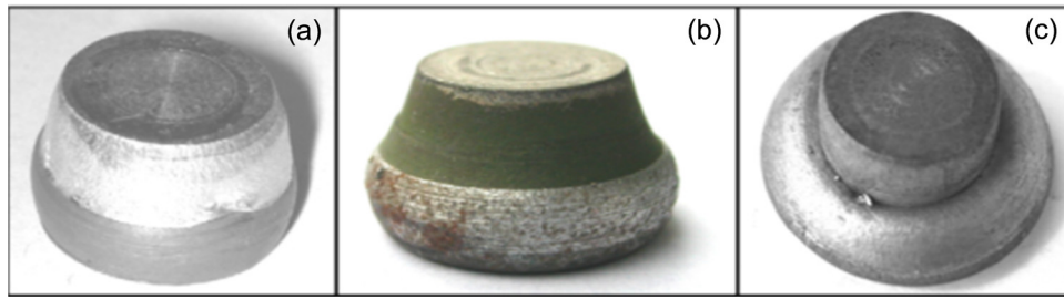
Fig. 3. Dissimilar metal preforms after hot compression to 50% reduction showing the effect of (a) small difference (Cu–Al), (b) intermediate difference (stainless steel–steel), (c) large difference (steel–cu) in flow stress between the base metals (Domblesky et al., 2006)
