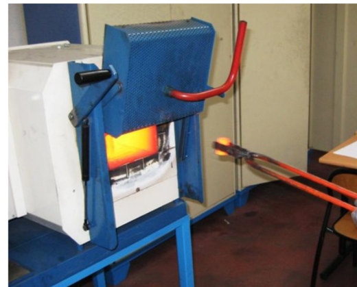
Fig. 6. Setup for experimental upsetting test, (a) upsetting setup and (b) furnace.
