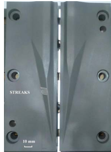
Figure 6. Flat dies used for the experimental tests
