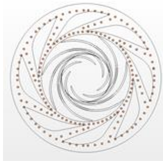
Figure 4. Probes for frozen rotor calculations.
