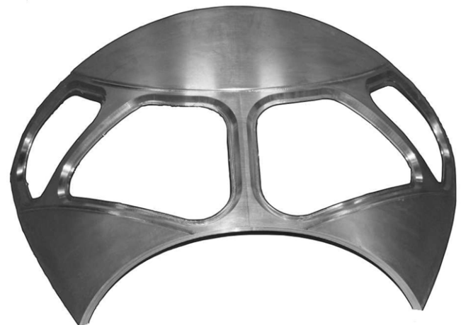
Fig. 9. Manufactured prototype of the cockpit.
