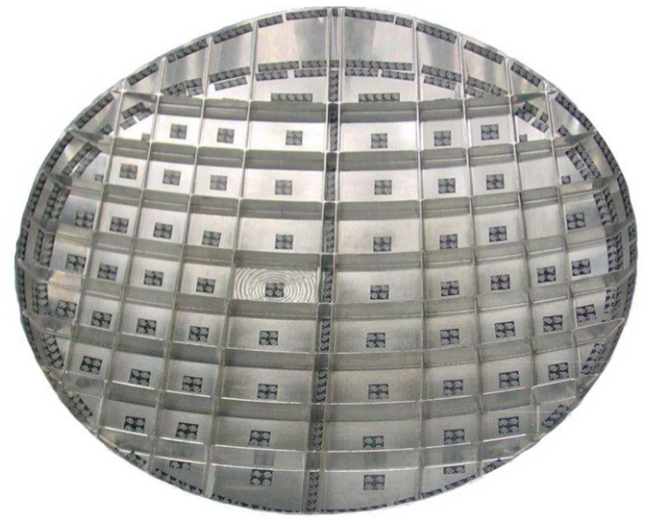
Fig. 7. Prototype of a forward pressure bulkhead.
