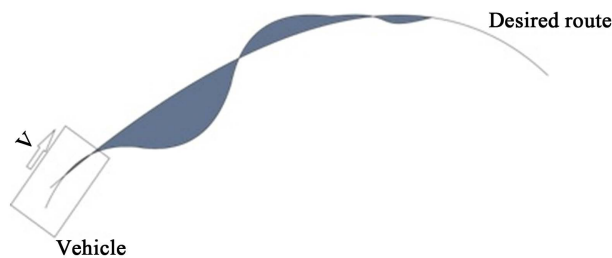
Figure 9. Lateral displacement area.
