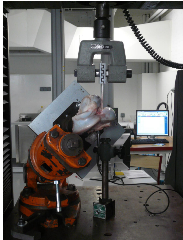
Fig. 3 ACLR loading experimental set-up
