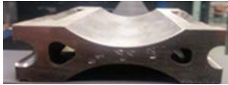
Figure 2. Rectangular specimen cut from cylinder liners
