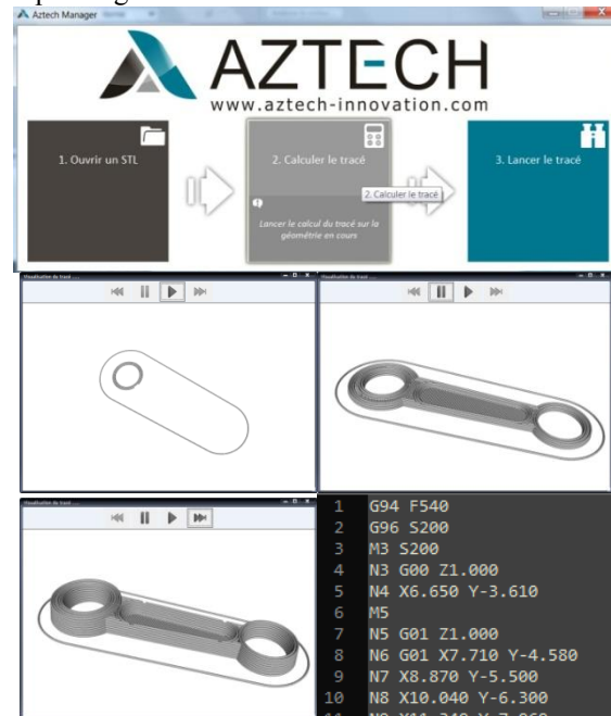
Fig 10. Additive manufacturing software for CNC machining and piston depositing system.
