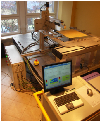
Fig. 2. Terahertz TDS spectrometer with scanning unit.
