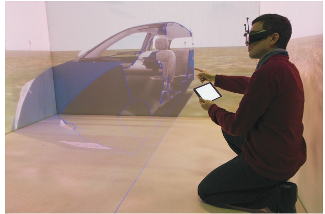
Figure 1: VARI 3 allows a user to explore and modify a single virtual vehicle model displayed simultaneously on both a CAVE and a tracked tablet.
